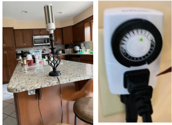
Figure 1: Portable ultraviolet light (UVC/UVA) lamp mounted on stand and set via timer for surface disinfection. Timer below kitchen counter is illustrative of the type shown here.
