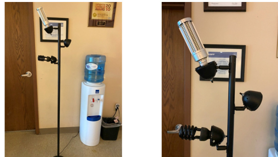
Figures 1a and 1b: UVC/UVA (black light) stand for office waiting room after-hours disinfection.
